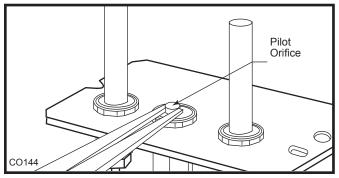
Fig. 12 Remove pilot orifice.
